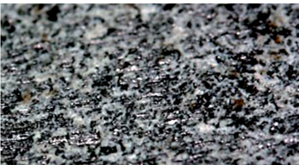
CC155 G8 surface with self lubricating Graphite particles
